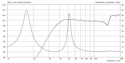
1) Drive voltage of 2.5Vrms chosen to provide 1W to the loudspeaker at 100Hz. Zmin=6.0 $\Omega$ , Znom=7.8 $\Omega$  from 35Hz to 120Hz. 2) 1012W @ 90Vrms / 8 $\Omega$  AES2-2013 2hr test. 1350W @ 90Vrms / Zmin=6.0 $\Omega$  AES2-1984(r2003) 2hr test.
